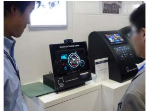
The naked-eye 3D display that tracks the movement of the head (left) and the curved display using an in-cell touch panel (right)
