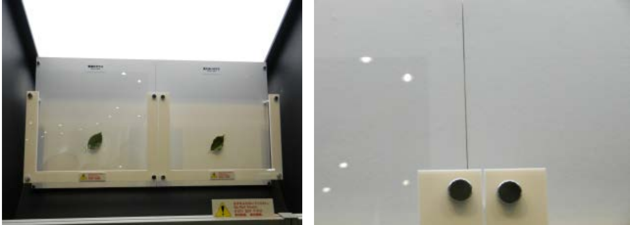
A normal glass substrate (left) and the new substrate (right). Because light is hardly reflected on the new substrate, it can hardly be seen; a close-up shot of the normal glass substrate (left) and the new substrate (right)
