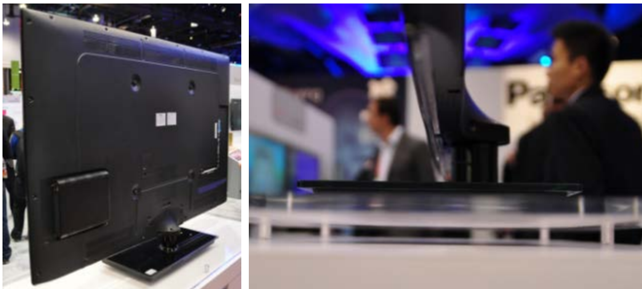
No cable is seen on the back side; A side view. The TV and the power-transmitting device are separated.
