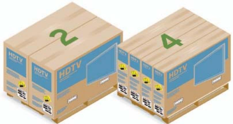
*Using conventional cushioning foam (left), a large flat-screen television can be packed with only two units to a standard pallet. ARCEL resin (right) allows for cartons approximately half that size, easily doubling the yield.*
