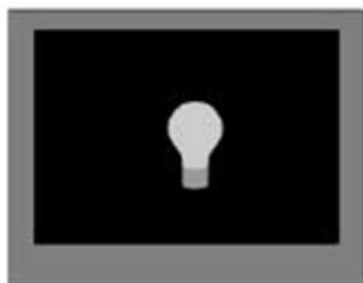
Specular (mirror like) reflection component only, a distinct image of the light source can be seen.
