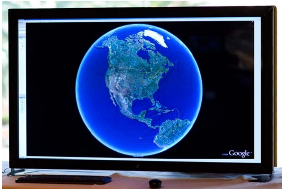
The Westinghouse D56QX1 is 56-inch display at 3840x2160 pixels is compatible with a wide variety of dual-link DVI video cards
