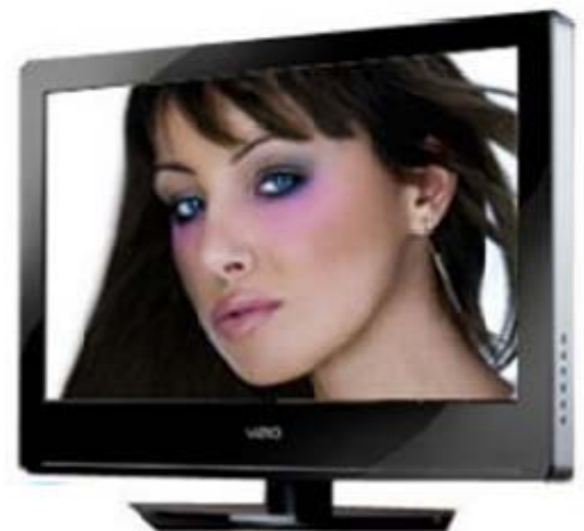
VIZIO's VA22LF is a 22-inch LCD TV at full-HD resolution of 1920x1080 pixels.
