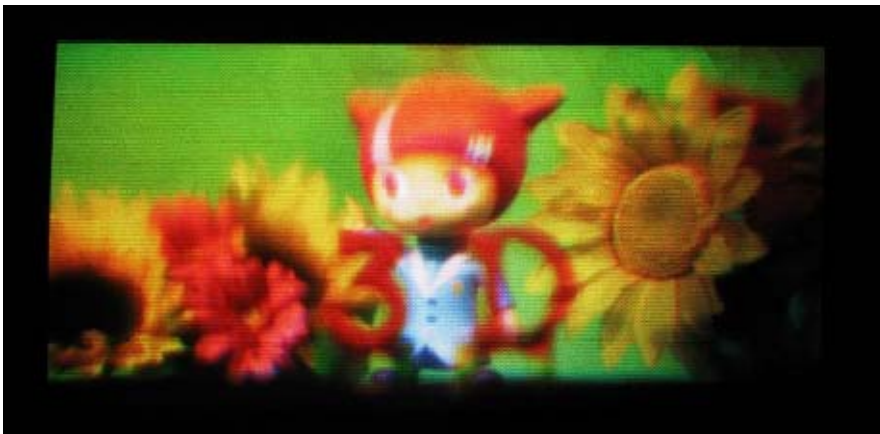
The 33-megapixel integral 3D display. The resolution of the 21-inch model is equivalent to 400x250.
