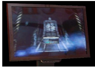
At CeBIT in March, Korea's Pavonine showed off their forthcoming 24-inch stereoscopic display, featuring 1920x1200 pixels. The MIRACUBE G240S is 2D/3D switchable with polarized glasses, (and so only supports 1920x600 pixels in 3D mode. No word just yet on pricing. The company is also reportedly preparing a 32-inch 3D LCD monitor. <u>http://www.dimen.co.kr</u>
