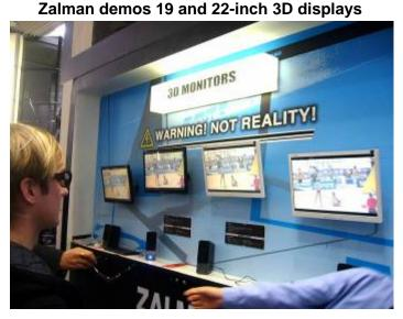
Zalman showed off two 2D/3D switchable monitors at CeBIT; one 19-inch 1280x1024 model targeted at gamers, and the other a 22-inch widescreen 1680x1050 model. Both of the displays require the user to wear glasses to combine the stereo images, although Zalman promises that the price of these monitors will undercut the competition.<u>http://www.zalmanusa.com</u>
