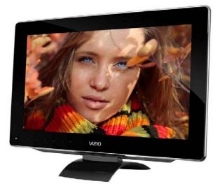
The Vizio 19" and 23" Razor LED LCD HDTV models use proximity sensing to activate the front panel touch controls.
